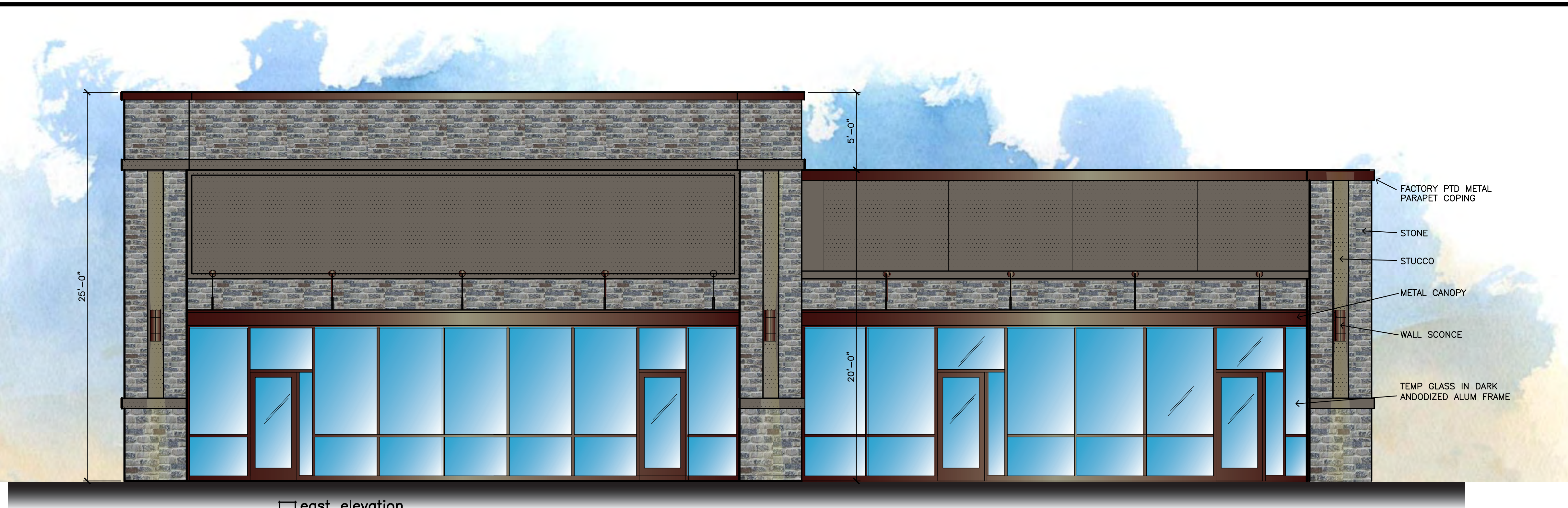
1 east elevation scale: 3/16" = 1'-0"
